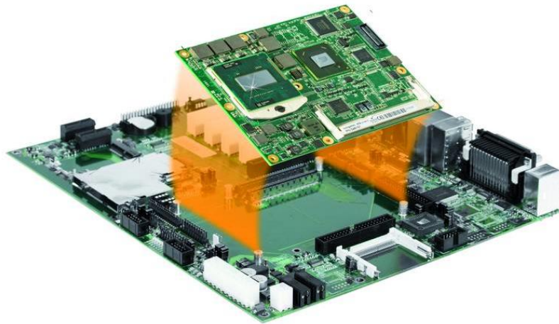
Figure II-4: Computer on a module
