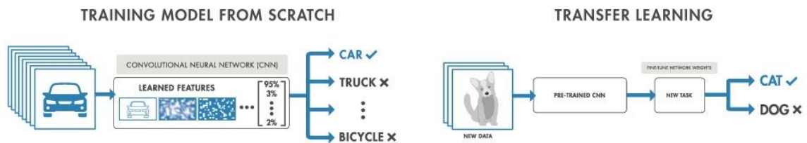
Figure I-30: Comparison of training a model from scratch and transfer learning. [16]
