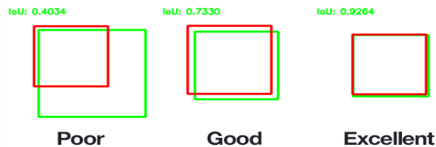
Figure III-3: e.g of computing IoU for various bounding boxes.
