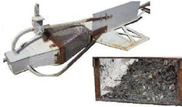
Figure 2 : nasse type Helley-Smith (Camenen et al., 2012)
