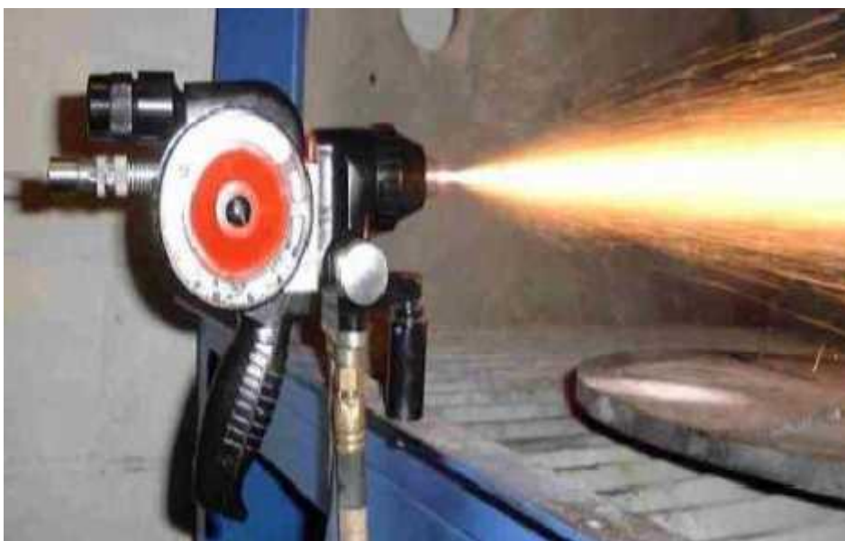
Figure II.9. Pistolet de projection a flamme fil [2-3].
