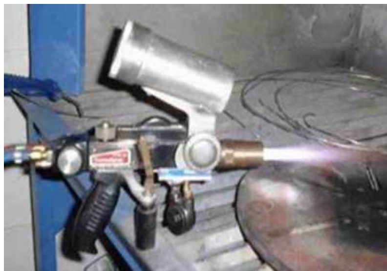
Figure II.7. Pistolet de projection flamme type 5PII [2-3].
