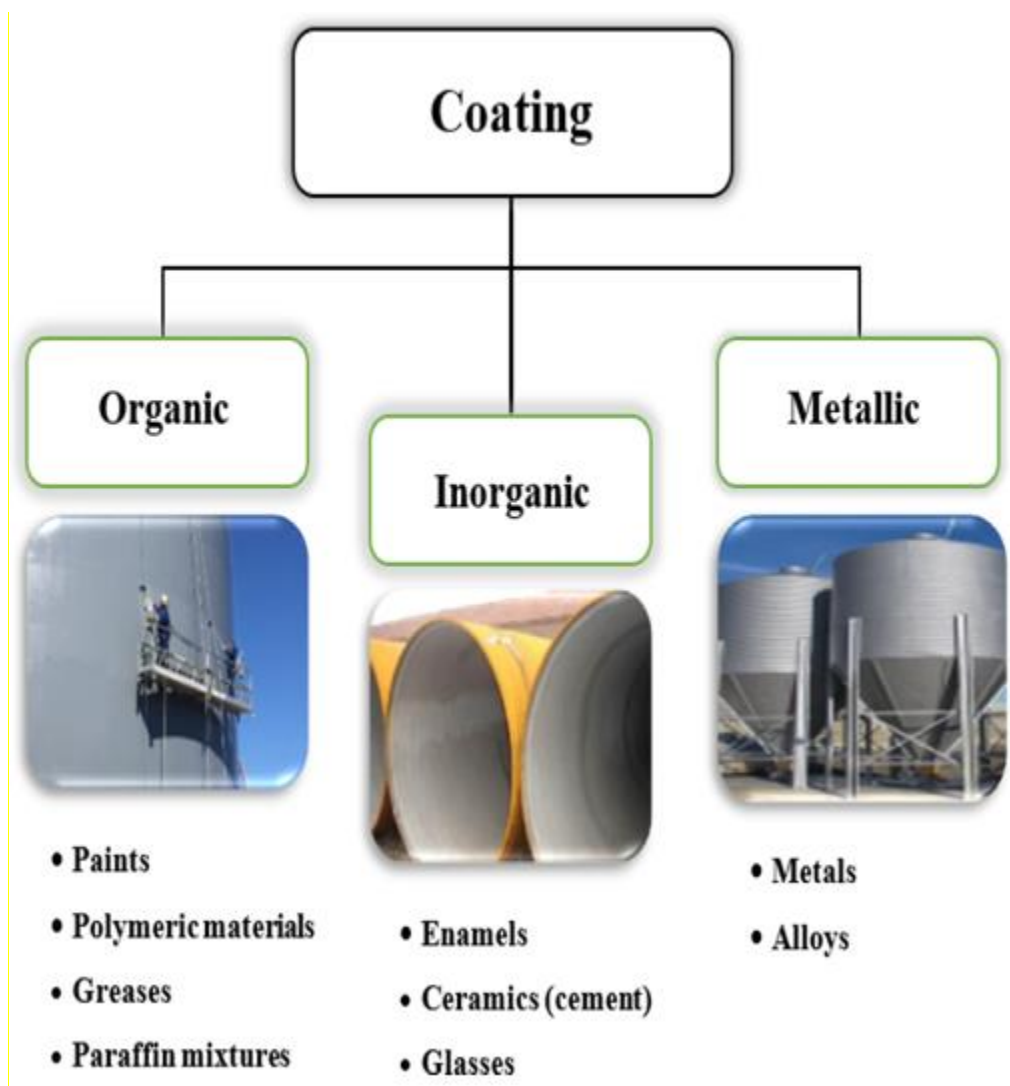
Figure.I.41. Different types of coating used in oil and gas industry .
