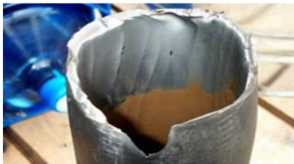
Figure IV.1: Oil and Gas pipeline after being attacked by Stress Corrosion Cracking
