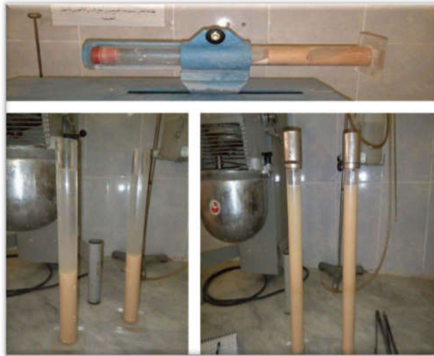
Photo II. 2 Essai Equivalent de sable
