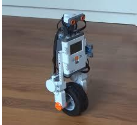
Figure I.2: LEGONXT-Based Self-Balancing Unicycle Robot Prototype [2].
