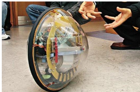
Figure I.3: Traditional Single-Wheeled Robot [3].
