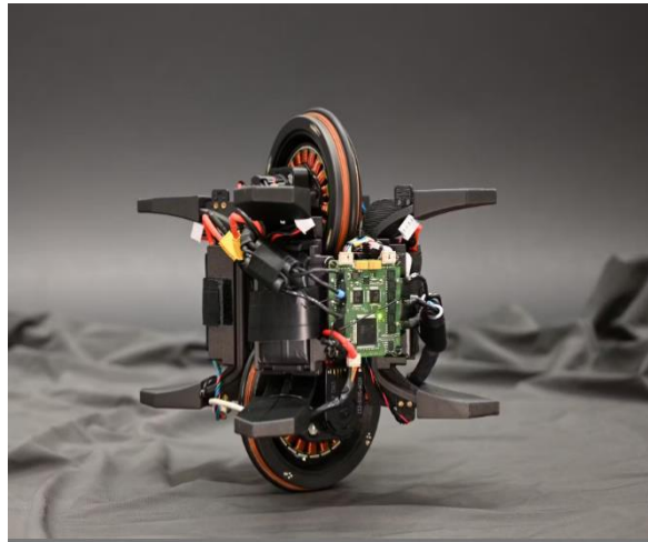
Figure I.4: Self-Balancing Single-Wheel Robot [4].
