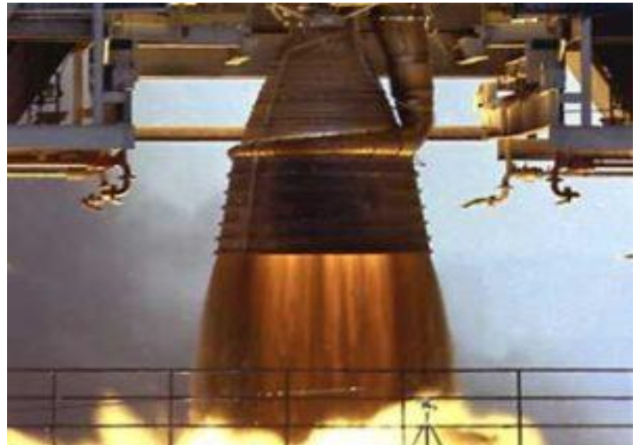
Figure.1-1 engines of a Saturn v rocket used both regenerative and film cooling to stay cool.
