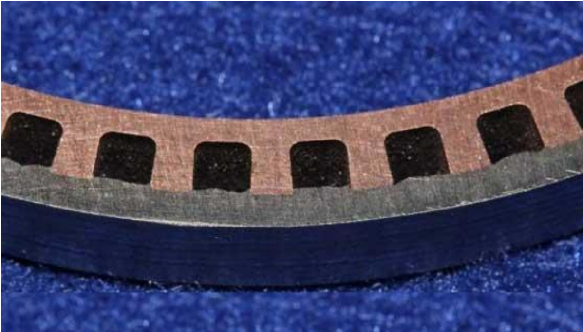
Figure1-3: a cross-section of a modern combustion chamber wall with the slotted liner, made from copper alloy, visible at the top with the structural jacket consisting of Inconel at the bottom.
