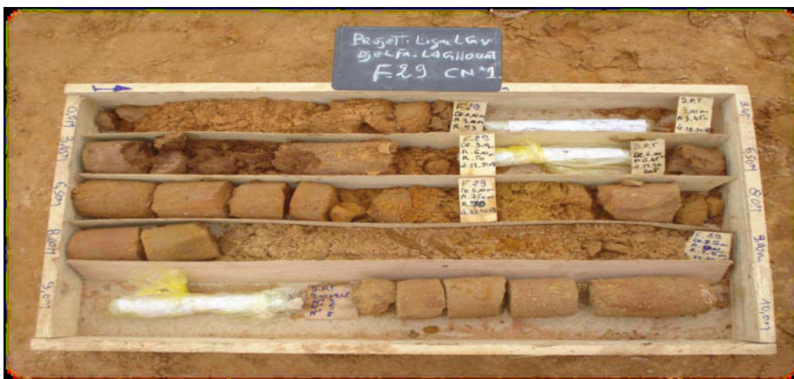
Figure III. 9 : Sondage S2- Caisse N°1 : 0.00 – 10.00 m
