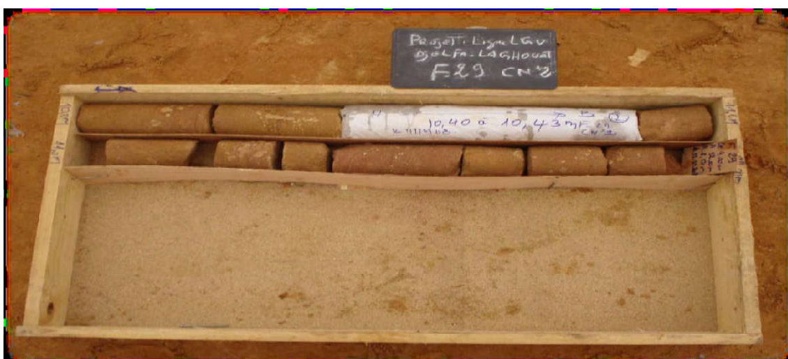
Figure III. 10 : Sondage S2- Caisse N°2 : 10.00 – 12.00 m
