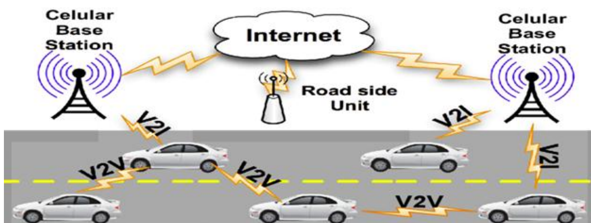
Figure 1.7: Hybrid communication in a VANET network [10]
