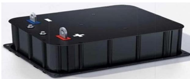
FIG I.22 –Example of a Supercapacitor
