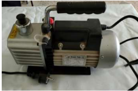
Figure III.22: Pompe à vide
