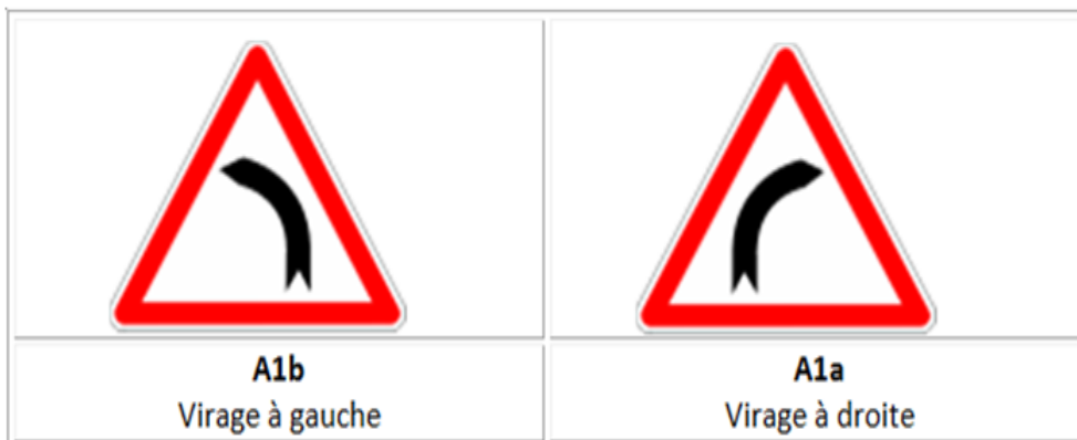
Figure V.5 : Signalisation vertical type A.
