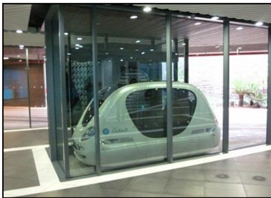
Figure I. 61 Personal rapid transit system. Source : http://www.archdaily.com
