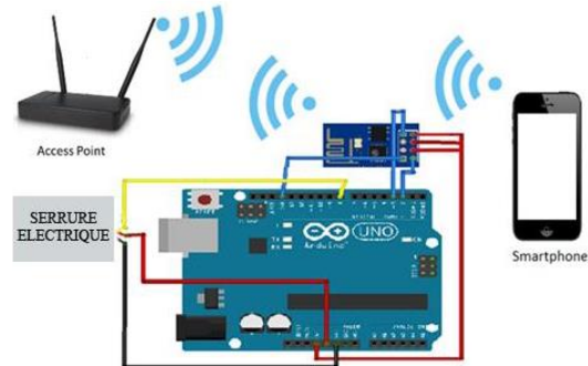
Figure 1. 10: Example of Esp8266 in microcontroller mode.
