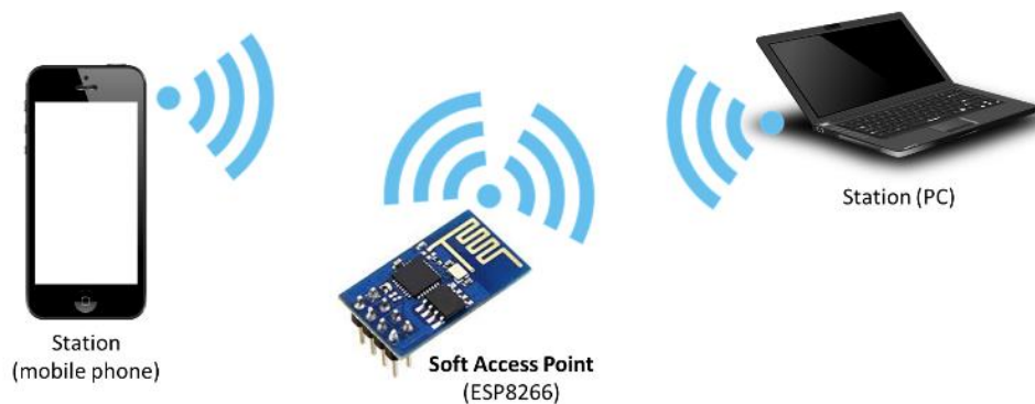
Figure 1. 12: Using ESP8266 in server mode.
