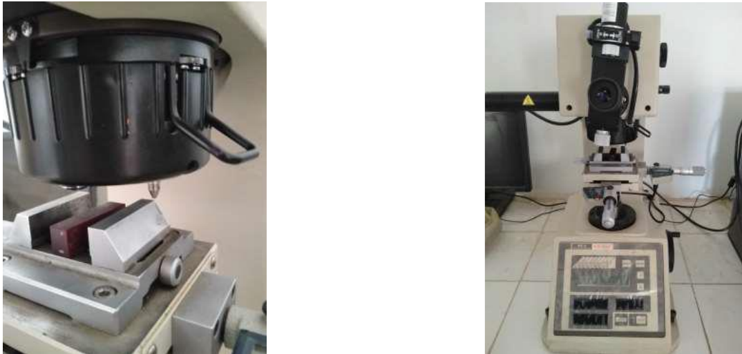
Figure. III.5: Durometer Model MVK-H2 (Hardness Testing Machine.)
