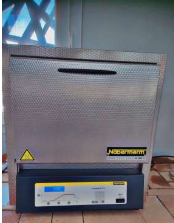
Figure 11: Four Nabertherm (labo mécanique)
