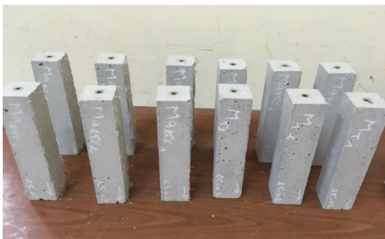
a. Specimens for free shrinkage
