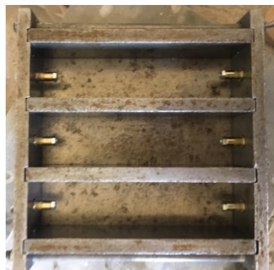
Fig.II. 25 Moulds for shrinkage test
