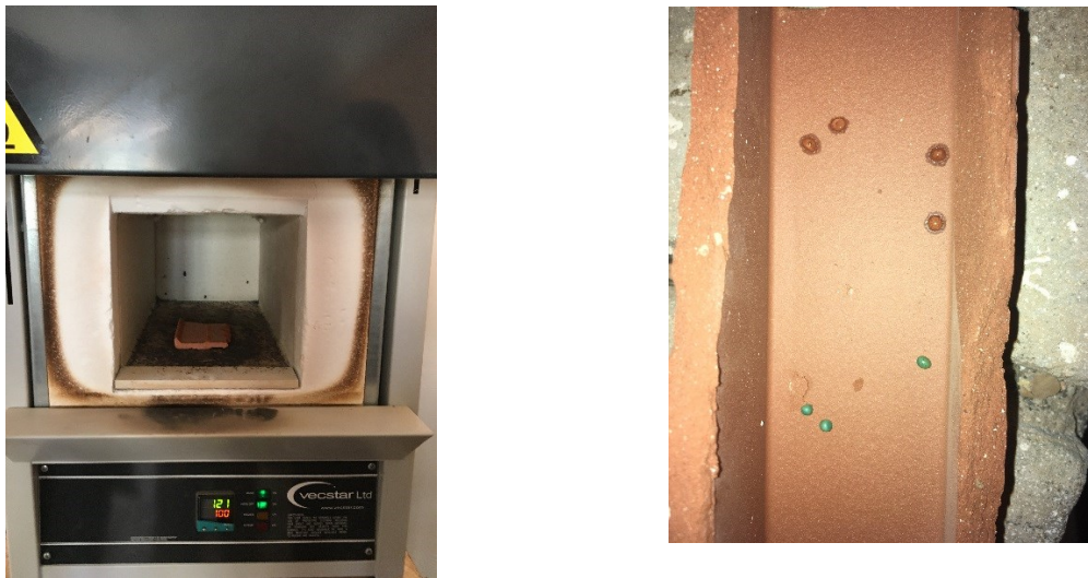
Fig.2. Melting temperature test of fibres
