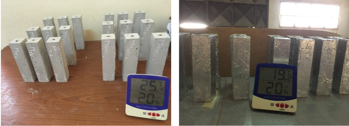
Fig.6. Measurement of temperature and moisture conservation
