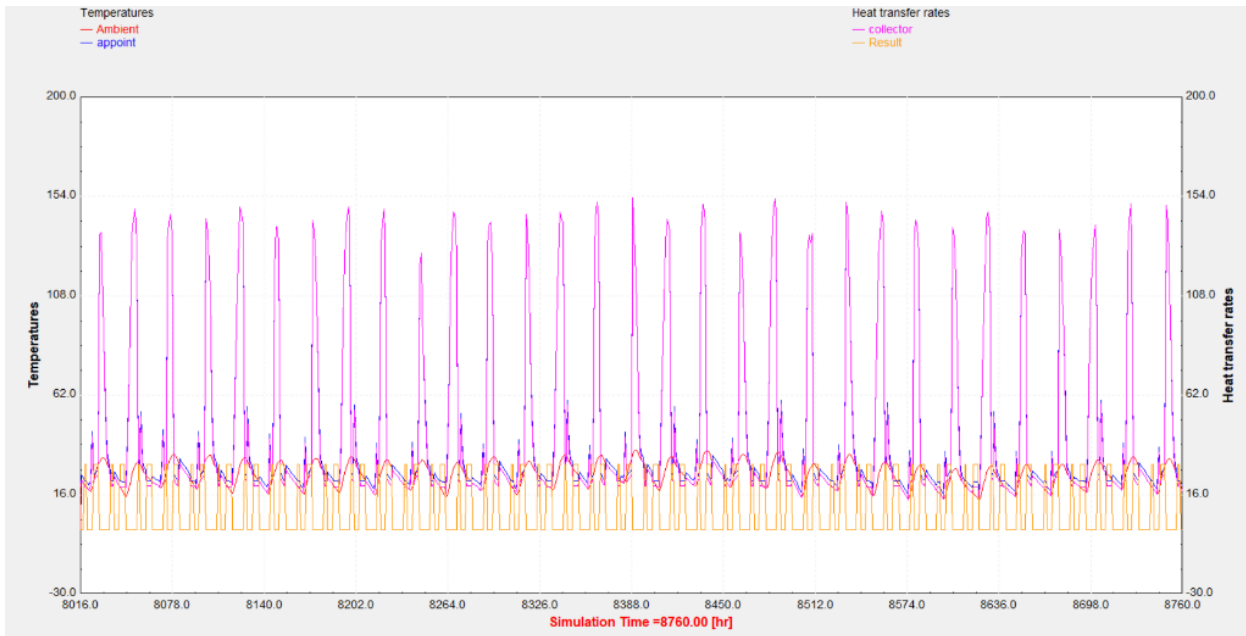
Figure V. 4: Overall TRNSYS response showing ambient temperature, control-related variable, collector behavior, and result/output over the simulated period.
