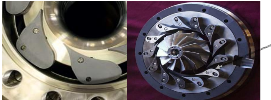
Figure I-7: Inlet Guide Vanes (IGVs)
