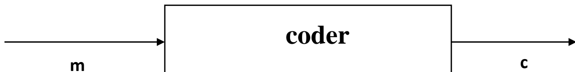
Figure II.2: Simplified diagram of a block encoder, which from an information word m of k bits, generates a code word C of n bits.
