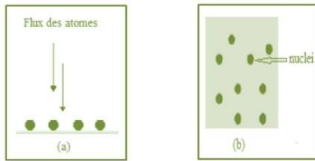
(a):the arrival of atoms on a substrate. (b): substrate morphology
