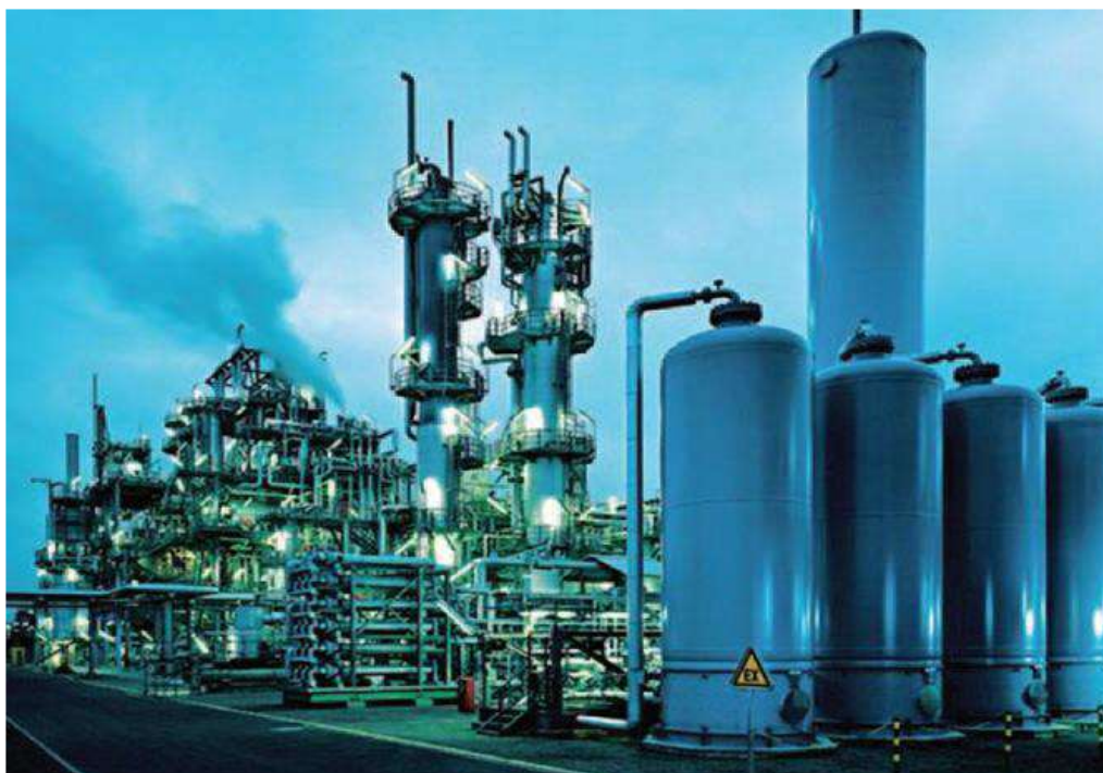
Figure 1.8 Hydrogen is co-produced with carbon monoxide from natural gas vaporeformation.
