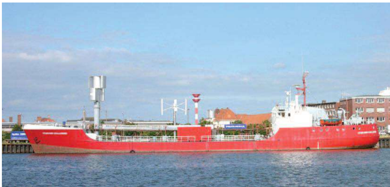
Figure 1.10 The Challenger ship, based in Germany, powered by a hydrogen engine produced by electrolysis powered by wind electricity.
