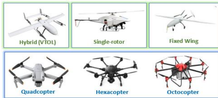
Figure 1.7: Different classes of UAVs based on wing types
