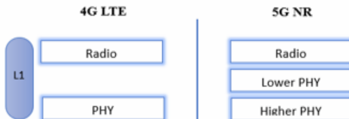
Figure 1.3: 4G LTE and the revised 5G NR in physical layer
