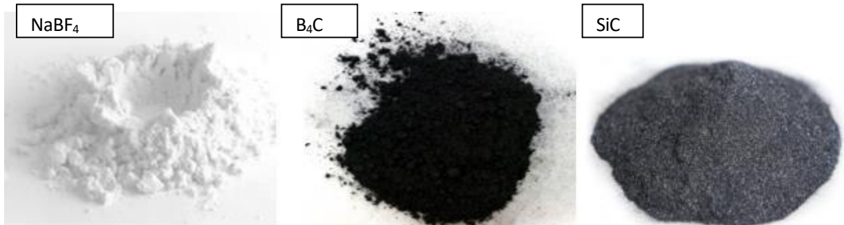
Figure 6 : Mélange de boruration (5% \text{NaBF}_4 + 5% \text{B}_4\text{C} + 90% \text{SiC} )
