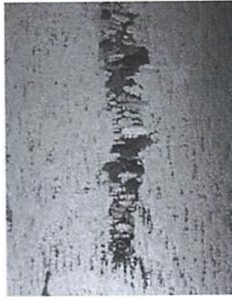
Fig.I.15: Freckle of 2 mm diameter, observed in a Ni super alloy [M. C. Schneider 58].
