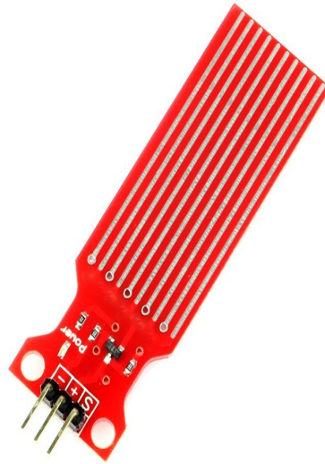
Figure 3.20: level water sensor
