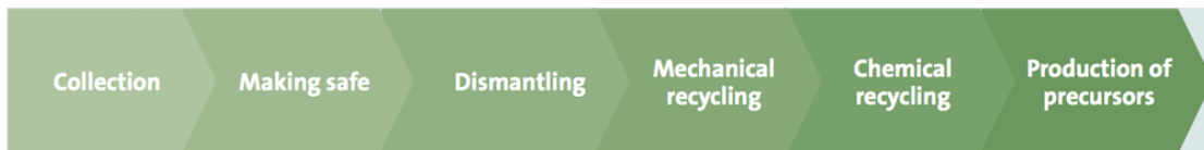
Figure III. 15 : Stages in recycling electric vehicle batteries
