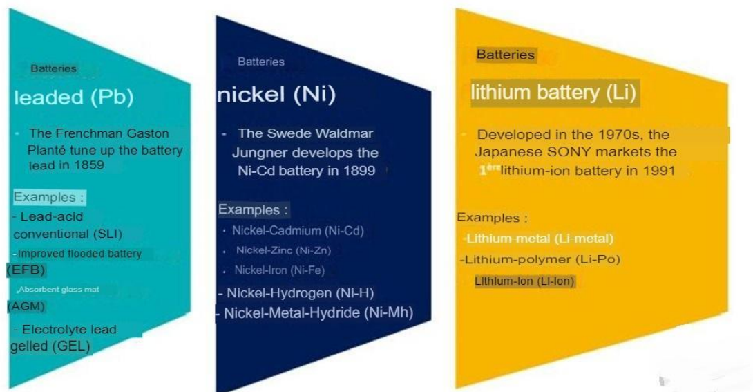
Figure I. 17 : Different type of materials in battery
