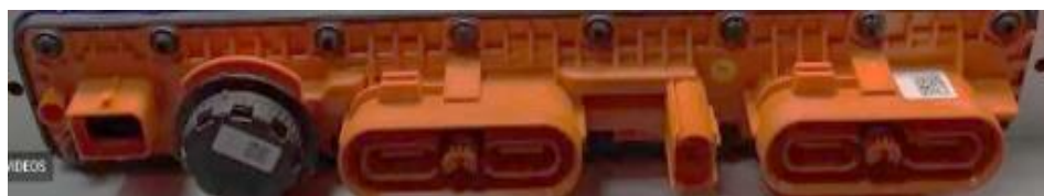
Figure I. 13 : High voltage connector strip [6]
