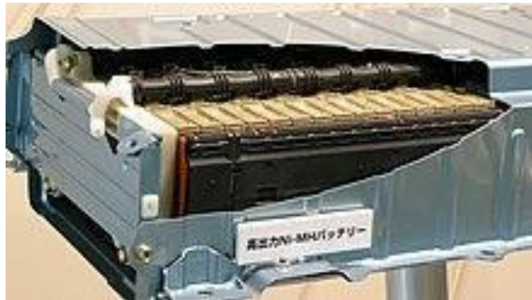
Figure I. 19 : High power Ni-MH battery of Toyota NHW20 Prius, Japan [10]
