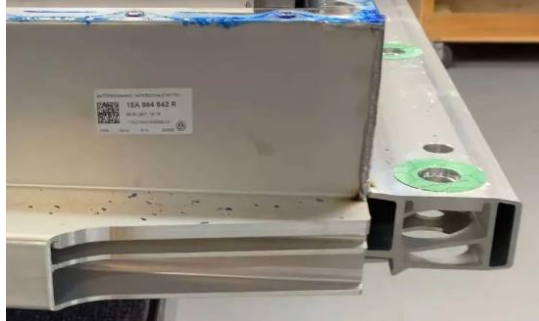
Figure I. 9 : Battery Housing side safety structures [6]
