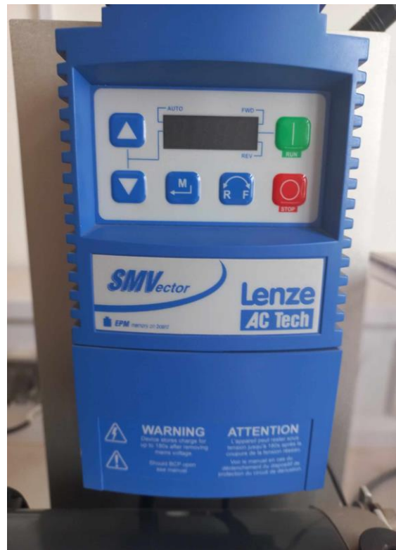
Figure 3.03. Variable frequency AC drive.
