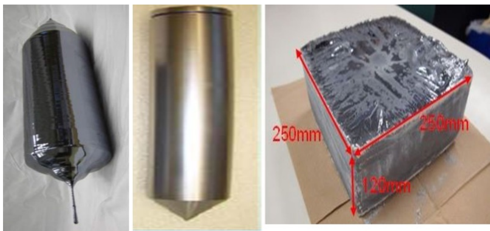
Figure 2.1: (a). Czochralski mono ingots, diameter: 800, length: 600 mm, (b). FZ mono ingot; (c). multicrystalline ingot [10].
