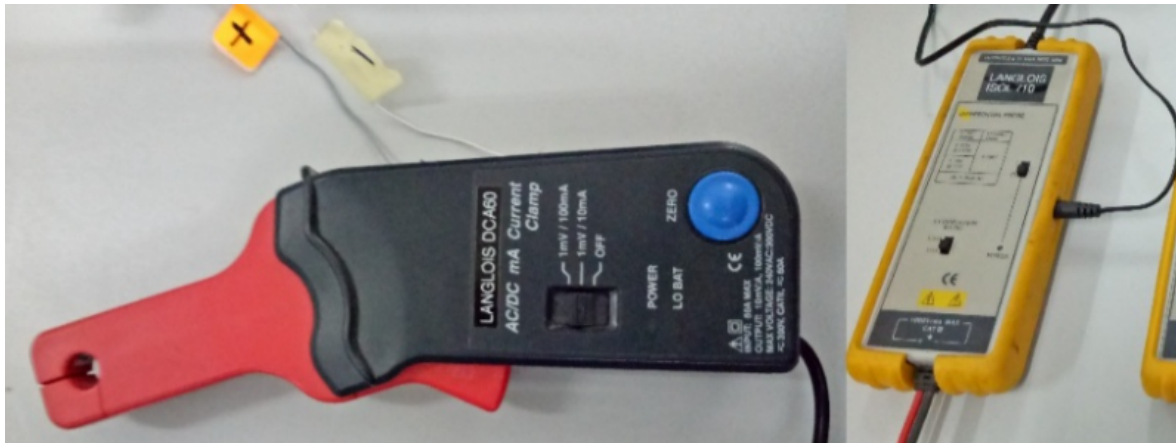
Figure 3.6: Current and voltage measurement sensors.
