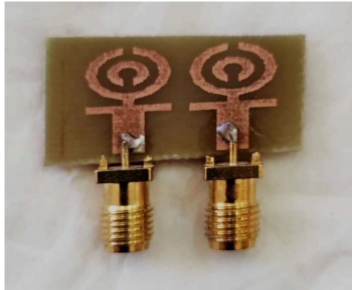
Figure 04: MIMO sensor (model 2: X3 in mm) with ports (front).
