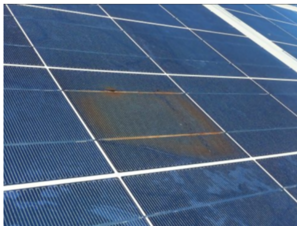
Figure 2.5: Discoloration of solar cell
