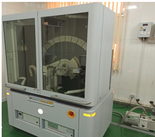
Figure I.5: Diffraction des rayons x (DRX).
