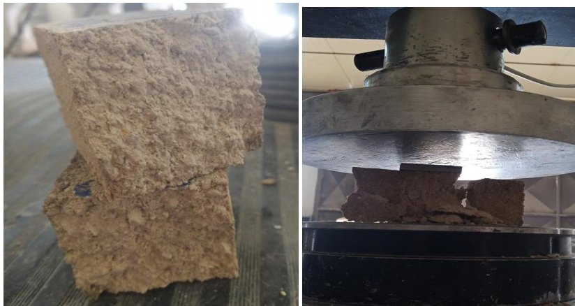
Figure II 21 : Essai de compression
