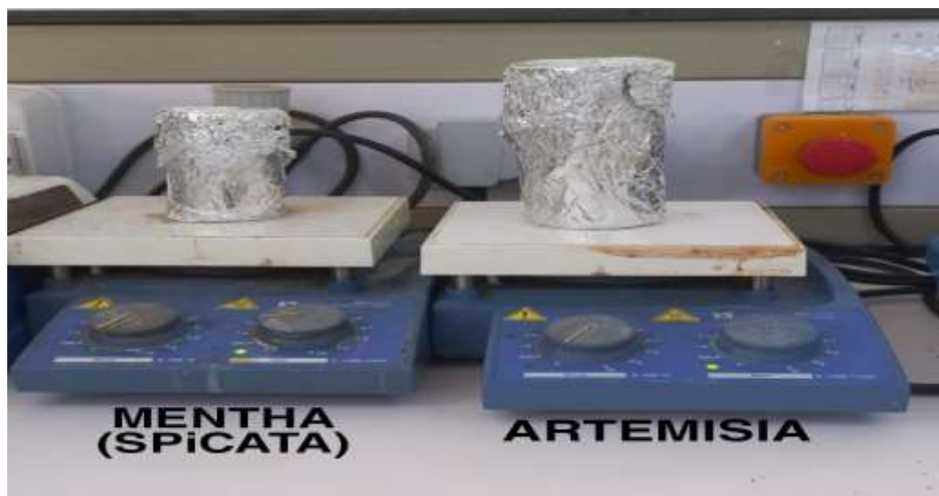
Figure III.5: Addition of extract to AgNO 3 to synthesize silver nanoparticles
