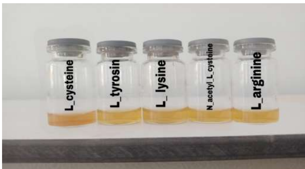
Figure.IV.8: Colorimetric Detection of Various Amino Acids Using AgNPs Synthesized from Mentha spicata Extract
