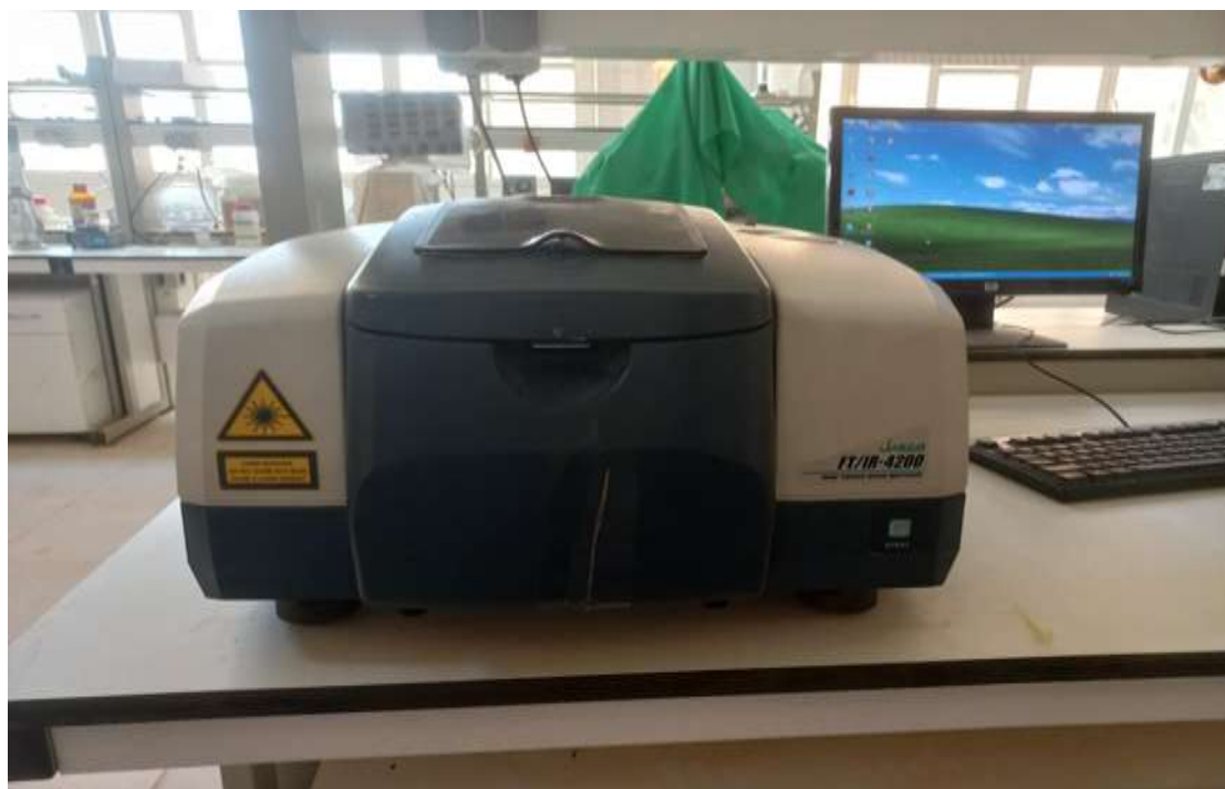
Figure III.13: Picture of FT-IR Spectrometer JASCO FT/IR4200.
