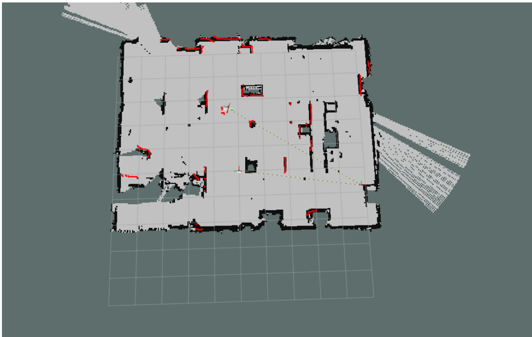
Figure 3.23: Real-time Mapping with GMapping and Loop Closure.
