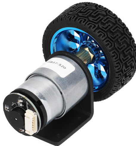
Figure 3.7: High power encoder motor.
