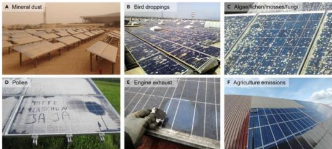
Figure I.25: Overview of various pollution photographs types by (A) mineral dust in a desert area, (B) bird droppings, (C) algae, lichen, mosses, and (D) pollen in wet and moderate climates, (E) engine exhaust from an industrial area, and (F) agriculture emissions [168].
