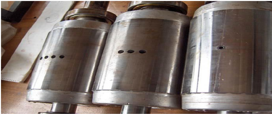
Figure 1.5 rupture de barre
