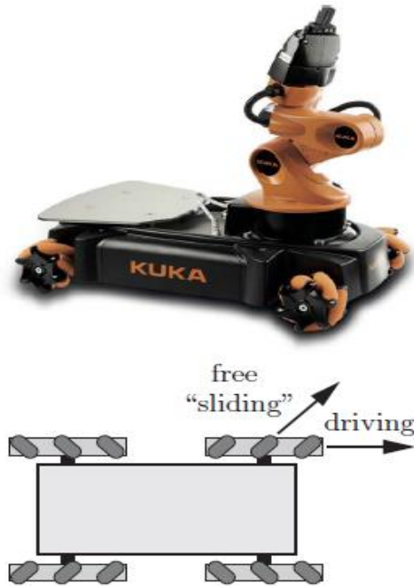
Figure 2.2: the Kuka youBot mobile manipulator system, which uses four mecanum wheels for its mobile base. [1]
