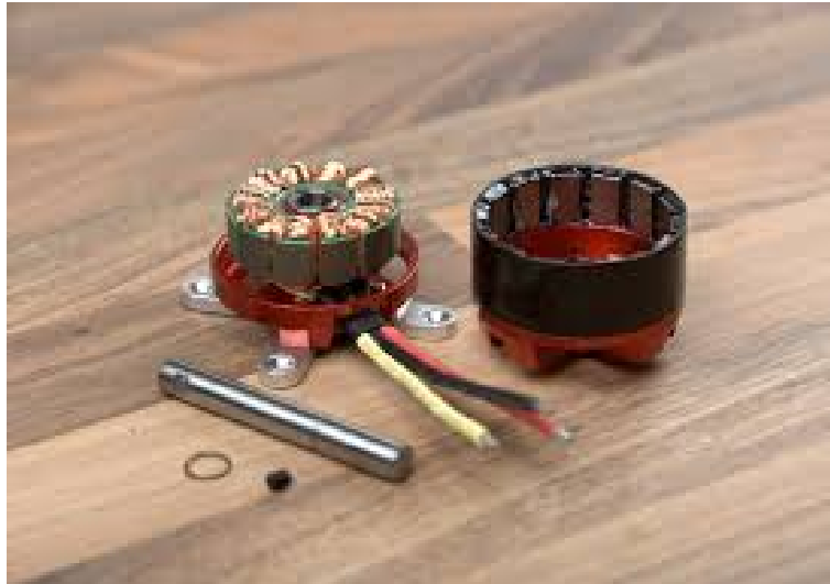
Figure 2.4: Outrunner brushless motor [38]
