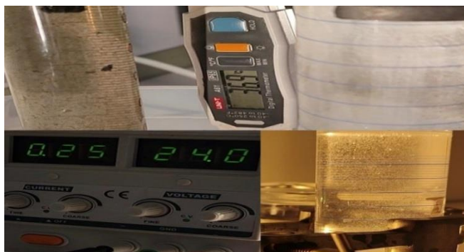
Figure II.6. The measurements of the produced gases during the water-splitting process
