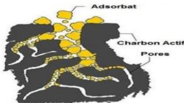
Figure I.1. Structure of an activated carbon [7]
