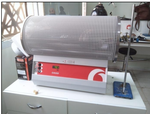
Figure 8. Tubular furnace used in the SAC regeneration process
