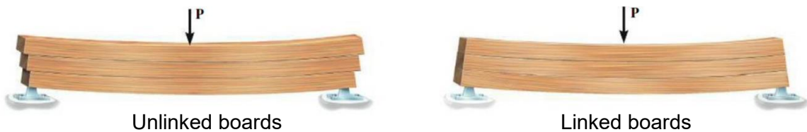
Figure 14. Illustration of the effect of bonding the plates on the longitudinal deformation of the fibers of beams in bending.
