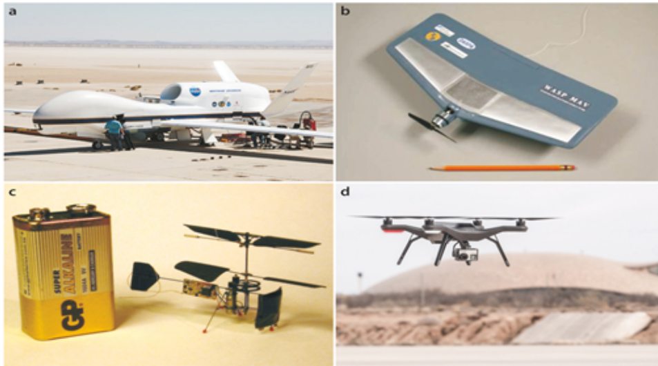
Figure 1.4: Flying robots. a) Global Hawk unmanned aerial vehicle (UAV) (photo courtesy of NASA), b) a micro air vehicle (MAV); c) a 1-gram co-axial helicopter with 70 mm rotor diameter; d) a quadrotor which has four rotors and a block of sensing and control electronics in the middle.
