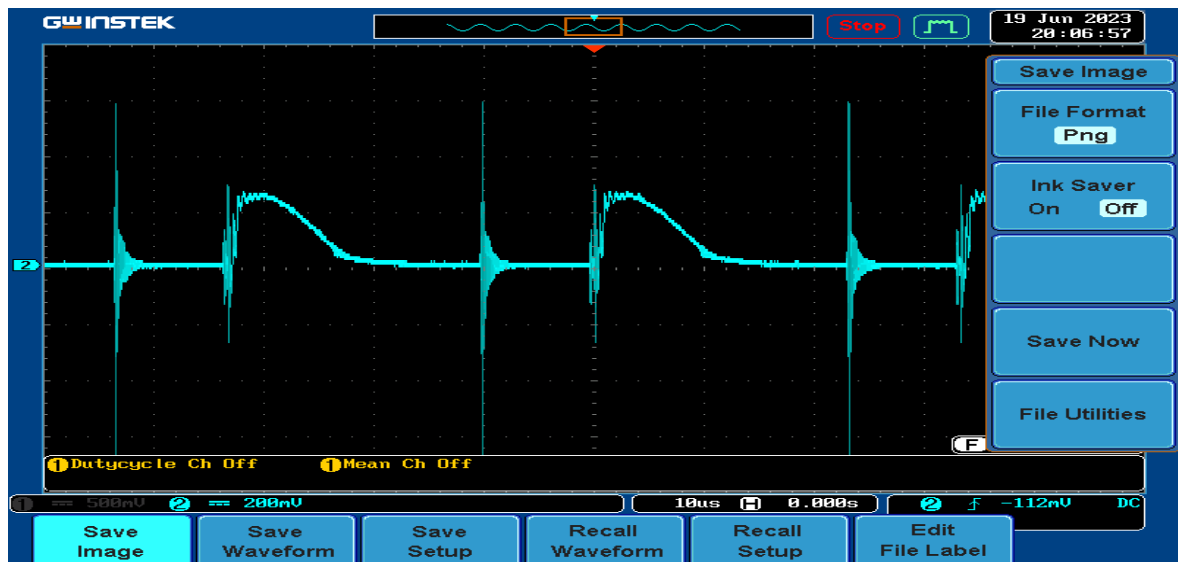
Figure III-25: Secondary winding current
