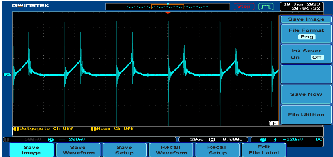
Figure III-24: Primary winding current
