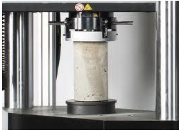
Figure II.33: Essai de compression.
