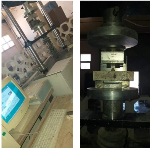
Figure III.18 : Essai de flexion simple.
