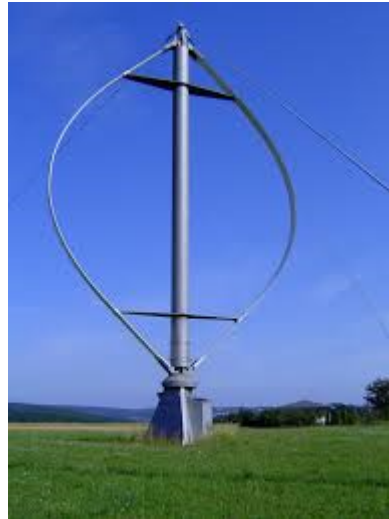
Figure 5.2: Vertical axis wind turbine.
