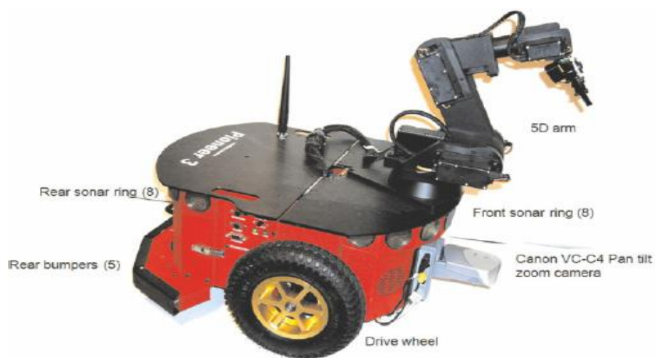
Figure I.7. Pioneer P3-DX sensors and actuators alternative configuration
