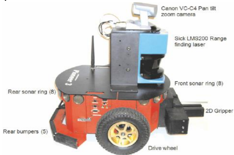
Figure I.6. Pioneer P3-DX sensors and actuators
