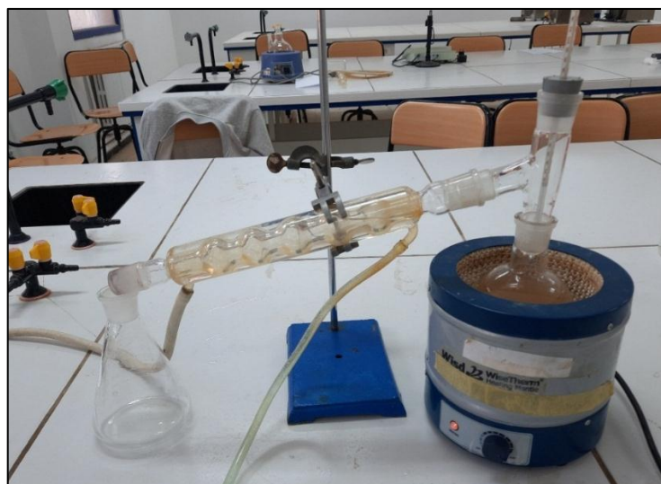
Figure 21: Distillation assembly for bioethanol production (Original photography, 2023)
