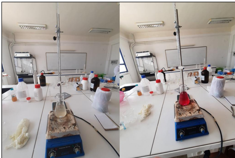
Figure 29: Total acidity titration (Original photography, 2023)
