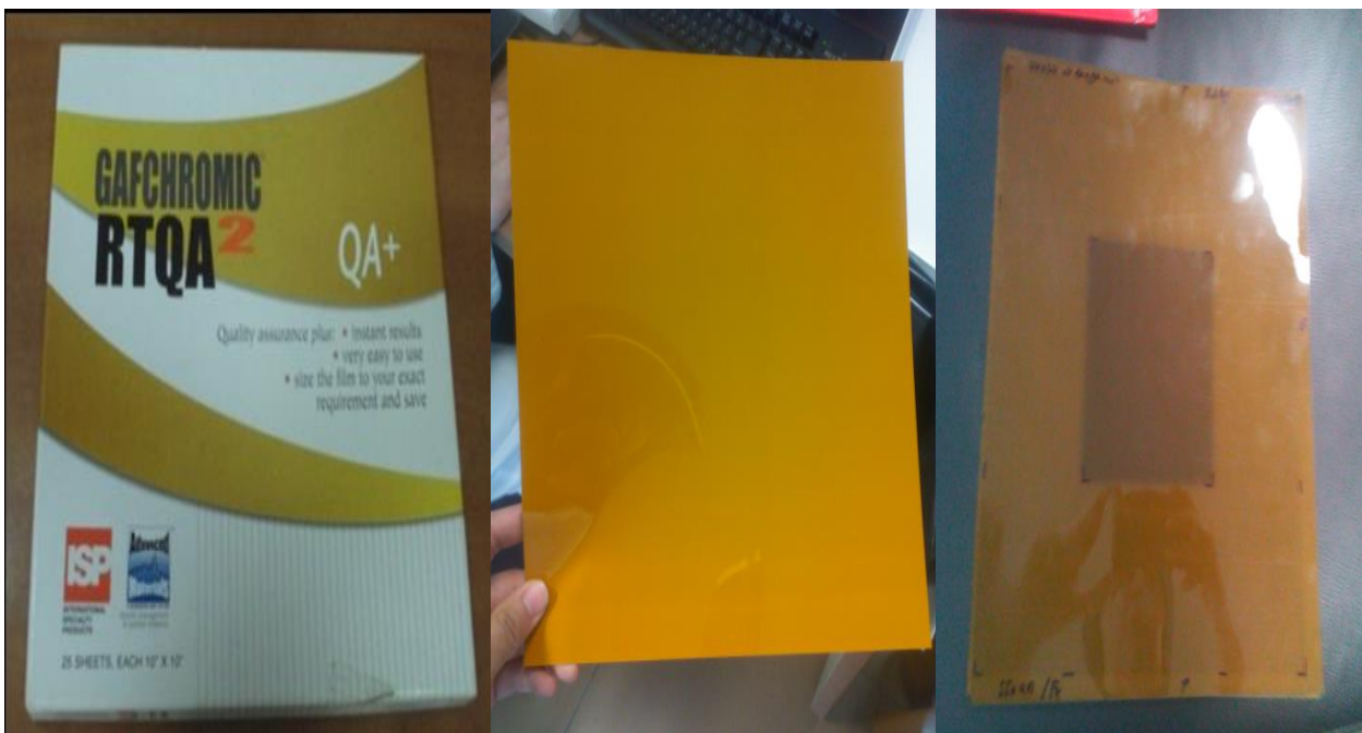
Figure III.5: Film chromatique [Centre Anti Cancer Athéna].
