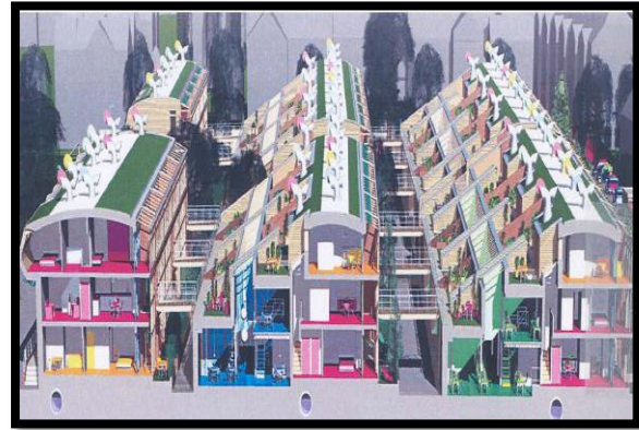
Figure N°31: la ventilation naturelle Source: http://www.cerdd.org/IMG/pdf/Bedzed_part1-2.pdf
